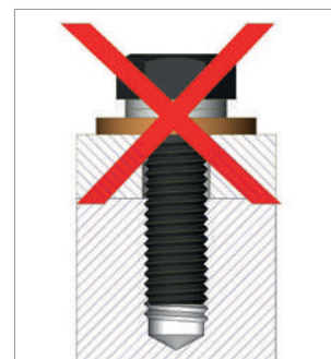
No locking function when combined with flat and freely rotating washers
